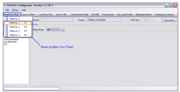
16 Figure Reading profiles from flash
