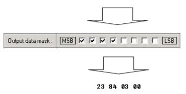
Data bytes are filtered by selecting the checkboxes in Output data mask. Note, that configurator has them listed starting with MSB.
