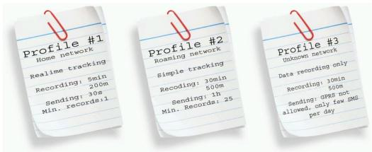
13 Figure Roaming application profile configuration example
