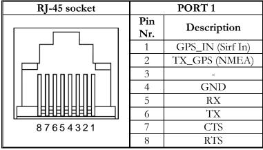
2 Figure RJ-45 Socket pinout
