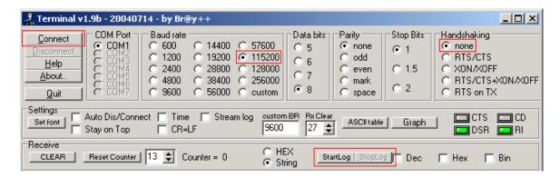
To debug NMEA GPS data, change baud rate value to 9600 and click connect.
