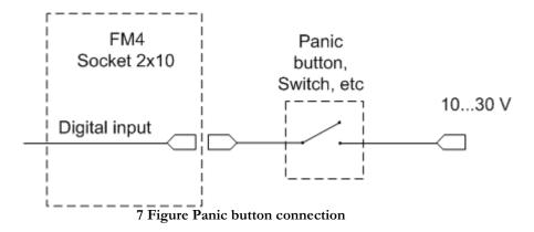
In cases when sensor output signal is negative an additional relay has to be installed to convert negative signal to positive.
