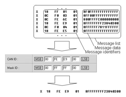
When certain message is filtered, FM4200 checks which data bytes should be sent to server. Document indicates that 5-8 bytes are used in FMS standard:
