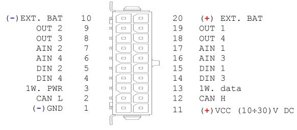
1 Figure Standard FM4200 2x10 socket pinout
