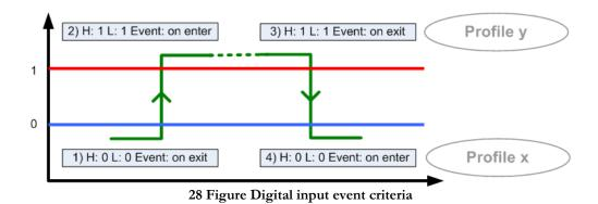
According to Figure, event on digital inputs could be described in different ways by using 1 and 3, 1 and 4, 2 and 3, 2 and 4 settings.
