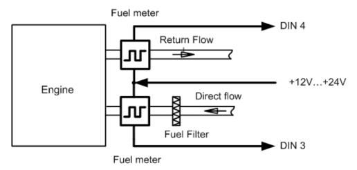
6 Figure Pulse fuel meters connection scheme
