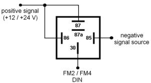
8 Figure Inverting relay connection
